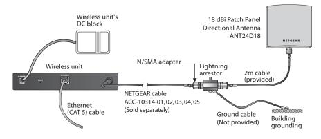
3. Connect the grounding cable (not included) from the lightning arrestor to the ground of the building.
